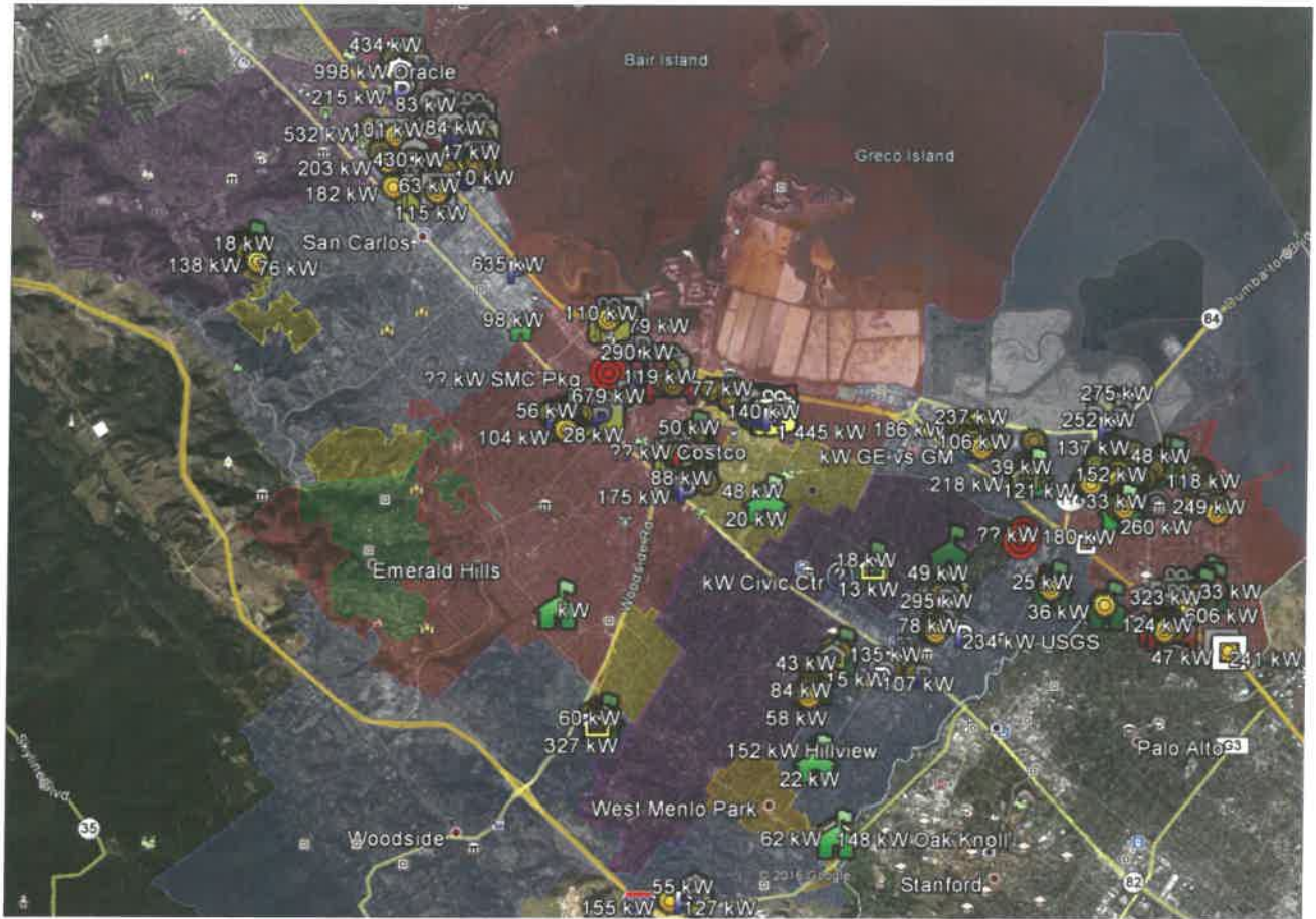
Figure 2- SSS Overview of Solar Siting Survey results for the Peninsula Advanced Energy Communities (PAEC) project
