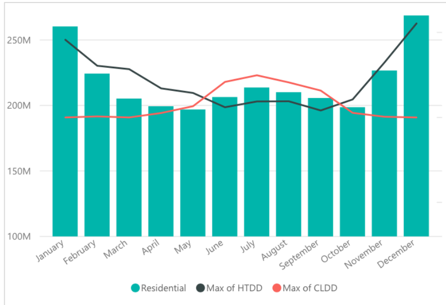
Figure 14: Analysis of monthly consumption (kWh) in EBCE's residential sector in relation to heating/cooling degree days. Note strong correlation between heating degree days and peak demand, indicating high usage of electric space heating equipment and opportunities for beneficial energy efficiency in the HVAC technology category.
