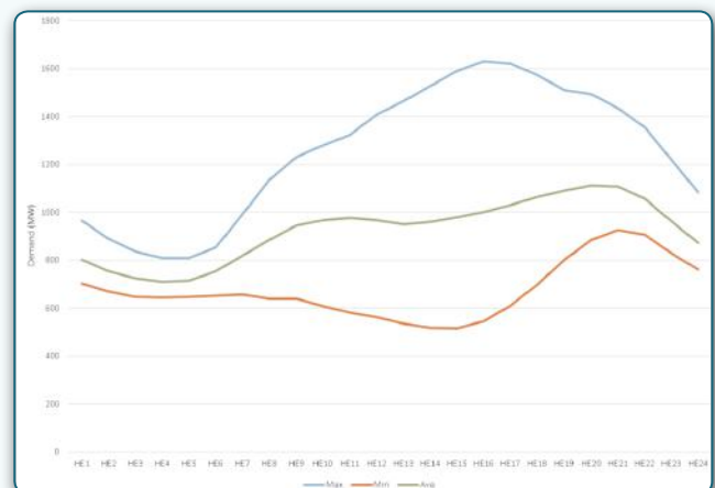
Figure 8: EBCE's annual hourly load curve (Maximum- top, Average- middle, and Minimum- bottom) in 2016. Note the emerging “Duck-curve,” which is less pronounced than the statewide averages.
