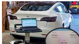
Tesla model 3 bidirectional charging test - Image credit Ambibox
